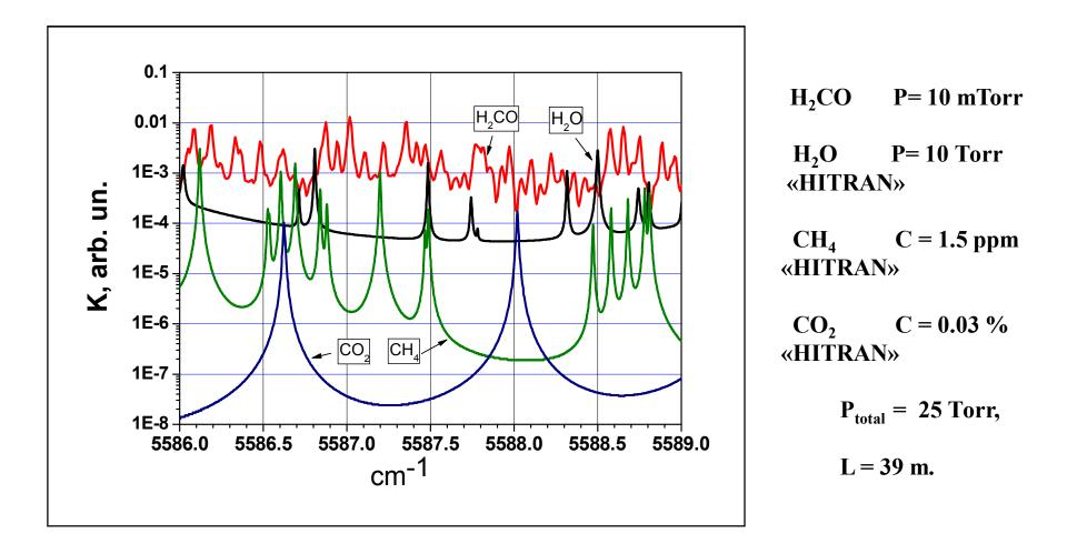
Analytical spectral range for  $H_2CO$  registration : 5586.7 – 5587.3 cm<sup>-1</sup> There are few interfering lines of gases:  $CO_2$ ,  $CH_4$ ,  $H_2O$
